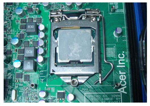
**IMPORTANT:** If you are going to install a new processor, note the arrow on the corner to make sure the processor is properly oriented over the socket.
